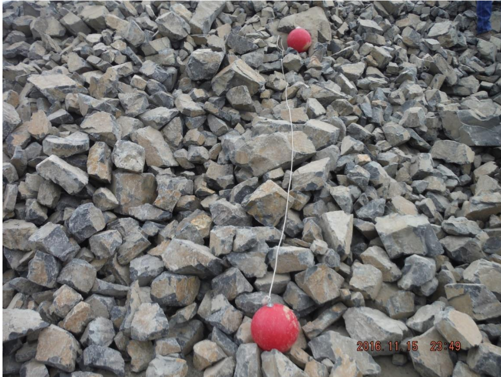
Figure 7 Zone 3A Drain Rock material stockpiled in November.
